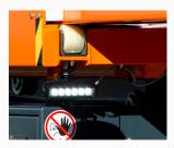
At all four corners a strong illuminated LED beamer is optional offered. Featuring a clear overall view of the surrounding area and working spot. These working light can be easy switch On and Off by a designated toggle switch at the upper or remote control box.
